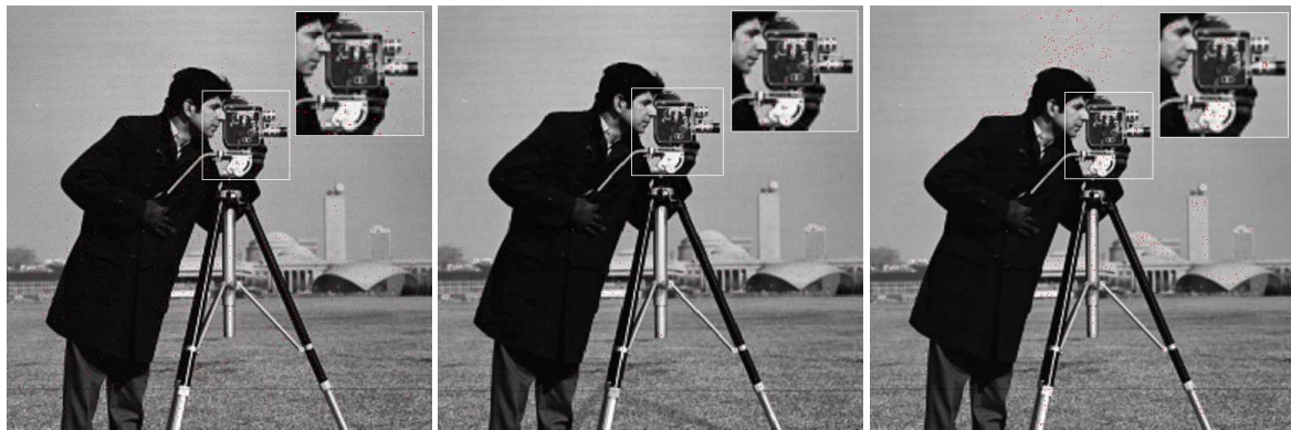
Figure 4: Bright key-points search in sharp and human posture images: from the left SURF result, SIFT result and CSA result.
