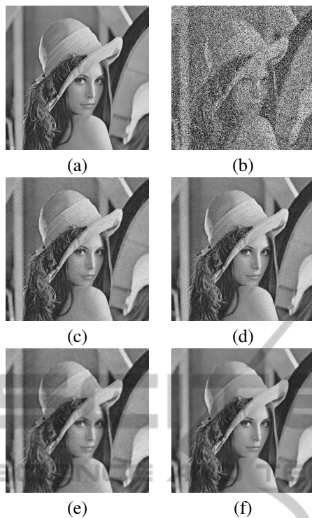
Figure 1: Denoising results of different algorithms on Lena image corrupted by noise variance ( \sigma=15 ) and impulse noise density ( p = 50\% ). (a) Original image, (b) Corrupted image, (c) TP (Jian et al., 2008), (d) FTPID (Jian et al., 2010), (e) AF, (f) Proposed Method.
