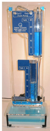
Figure 1: Real Coupled Water Tank System from Quanser.
