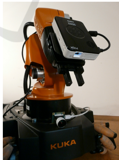
Figure 1: An LED pico projector AXAA P2 Jr mounted on the KUKA youBots manipulator and a uEye camera UI-1241LE-C-HQ on its platform.
