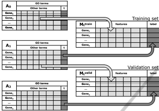
Figure 2: Illustrative diagram of the dataset representation for the prediction model of the annotations to a term t . The training set ( \mathbf{M}_t^{train} ) is created with an older annotation version \mathbf{A}_0 for the features and the current annotation version \mathbf{A}_1 for the labels. Similarly, the validation set ( \mathbf{M}_t^{valid} ) is created using \mathbf{A}_1 and a future updated annotation matrix \mathbf{A}_2 .
