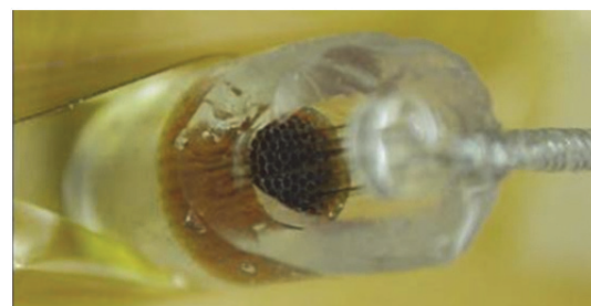
Figure 2: Magnified view of 3mm long, 203 \mu\text{m} diameter MicroTubes (brown) with 50 \mu\text{m} diameter insulated iridium microelectrode shafts placed halfway into 12 of the MicroTubes. The portal visible at the center of the picture is the exit port required for axon growth. Reference electrode coils and nerve cuffs were added to both the entry and exit chambers after this photo was obtained).
