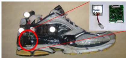
Figure 1: Shoe with IMU and Jig for facilitating ground truth capture using the Vicon Motion capture system.
