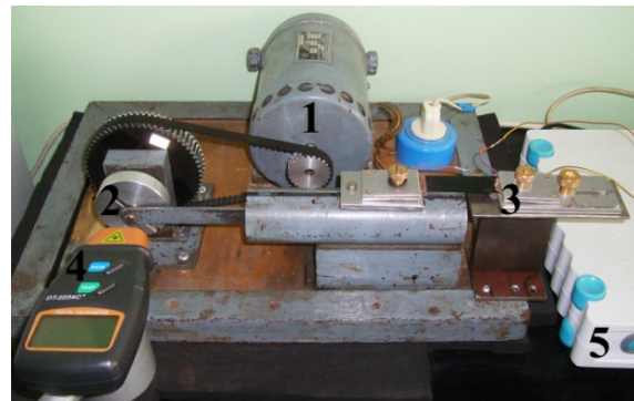
Figure 2: Equipment used for dynamic mechanical loading for low (top) and high (bottom) frequencies; where 1 – electric motor; 2 – eccentric sheave; 3 – sample; 4 – stroboscope; 5 – HBM spider 8. (cont.)
