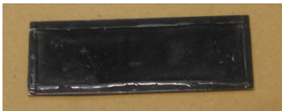
Figure 1: The clevios based sensor (glass support).
