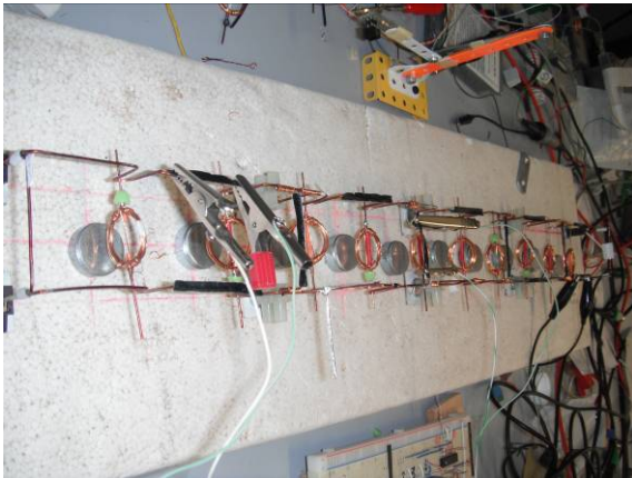
Figure 12: The complete electromechanical structure, with coils, magnets and the clevis based vibration sensors positioned on some sections of the structure.
