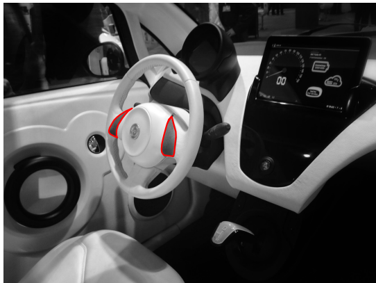
Figure 2: Integration of an Off-the-person ECG sensor into the steering wheel of a car; the electrodes are highlighted in red.
