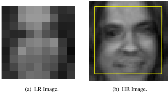
Figure 2: (a) The LR face image with size of 9 \times 9 . (b) The estimated HR image with size of 50 \times 50 .
