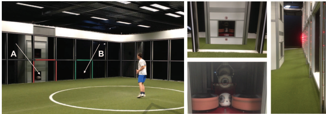
Figure 1: Footbonaut with testzone, ball throwing machines (A), target panels (B) and detailed view of ball throwing machines and light barriers.
