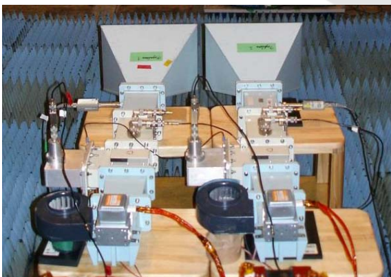
Figure 4: Photograph of a PVPCM phased array. The phased array was composed of two PVPCMs.
