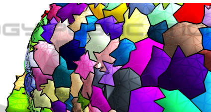
Figure 3: Surface triangles of the mesh of shoot apical meristem cells built from the tetrahedral mesh generated by Delaunay refinement.
