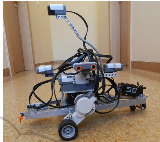
Figure 11: The construction of our robot - the robot is based on an aluminium frame (designed by (Artiemjew, 2014)) ; we have used Lego Mindstorms NXT bricks; there are four sonar sensors, a magnetic compass and a touch sensor; there are two HiTechnic sensor multiplexers - the first for digital and the second for analog sensors; there are two servo motors in use.
