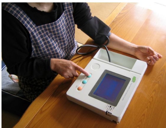
Figure 1: Snapshot in measurement of blood pressure using the device at home. The measured data were transmitted to a database server via a village network connection.
