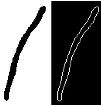
Figure 10: The shadow of a typical fibre particle (left) along with its boundary (right).
