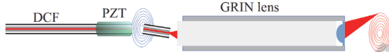
Figure 8: Complete scheme of the endomicroscope distal end containing the DCF to guide the excitation and collection signals, the PZT for scanning and the GRIN lens for the focalization and the collection.
