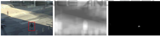
Figure 1: Influence of the \alpha parameter of the likelihood function. From left to right: the original image (the model is the histogram of the region surrounding the person on middle bottom), likelihoods maps with \alpha = 1 and \alpha = 100 .
