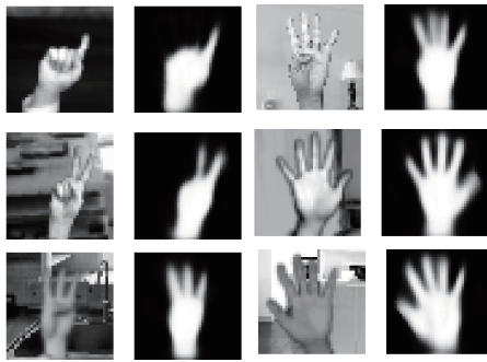
Figure 6: Output of binarization layer: the 1st and 3rd columns are original images and the 2nd and 4th are output images.
