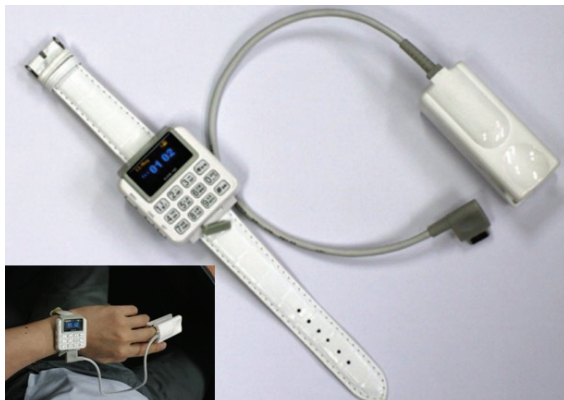
Figure 1: The illustration of our monitoring device.
