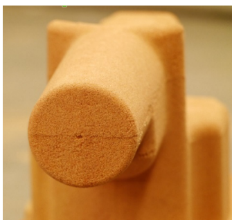
Figure 12: Sand core with simple shape and sand structure.
