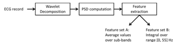
Figure 3: Feature extraction process of the spectral parameters.
