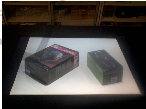
Figure 10: One image of a stereoscopic pair being presented over an horizontal display. This picture gives the idea of the user perception.
