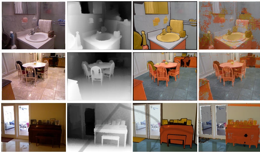
Figure 5: Image labeling examples on NYU Depth v2 dataset. Left to right: RGB image, depth visualization, ground truth, random forest segmentation.
