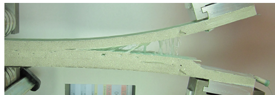
Figure 1: Fibre bridging phenomenon in a fibre reinforced polymer specimen.
