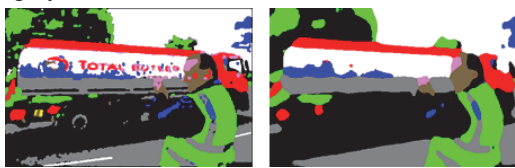
Figure 4: Left image is the result by applying a 3 \times 3 filter ten times. Applying the small filter many times does not decrease the number of regions much. Right image is the result by applying a 21 \times 21 filter once. The large filter loses the fine edge. For example, sky and the window of the truck become together.
