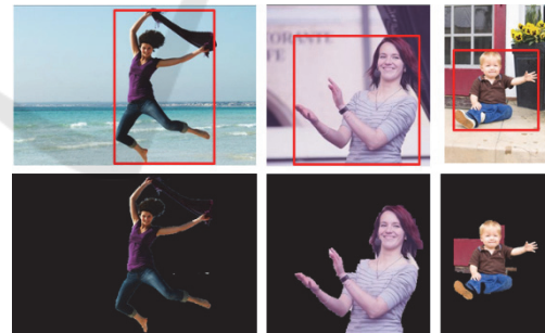
Figure 1: Top row shows positive training images. The red rectangle is the bounding box. It also includes background region. Bottom row is the segmentation results using the GrabCut. If we represent only the segmented human by BoW, the bad influence by background is reduced and the accuracy will be improved further.
