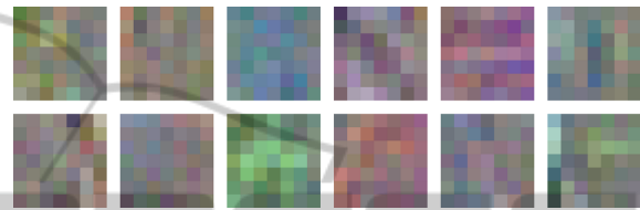
Figure 4: Convolution masks of the first layer found during learning on the KITTI road detection dataset.
