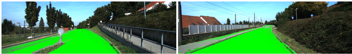
Figure 5: Qualitative results on the KITTI road detection dataset. Images show original input-data with labeled road pixels as green overlay. Although a spatial prior is used in our approach we are able to segment road scenes with curves or occlusions well. This figure is best viewed in color.
