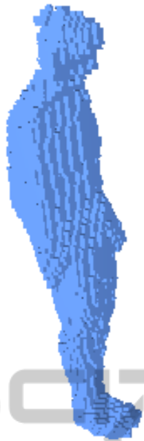
Figure 5: 3D reconstruction based on the input images of figure 4. The complete person is reconstructed while only 4 out of 7 cameras could see the complete person. Voxel size is 2cm x 2cm x 2cm. The traditional algorithm only reconstructs a few voxels from the head of the person.
