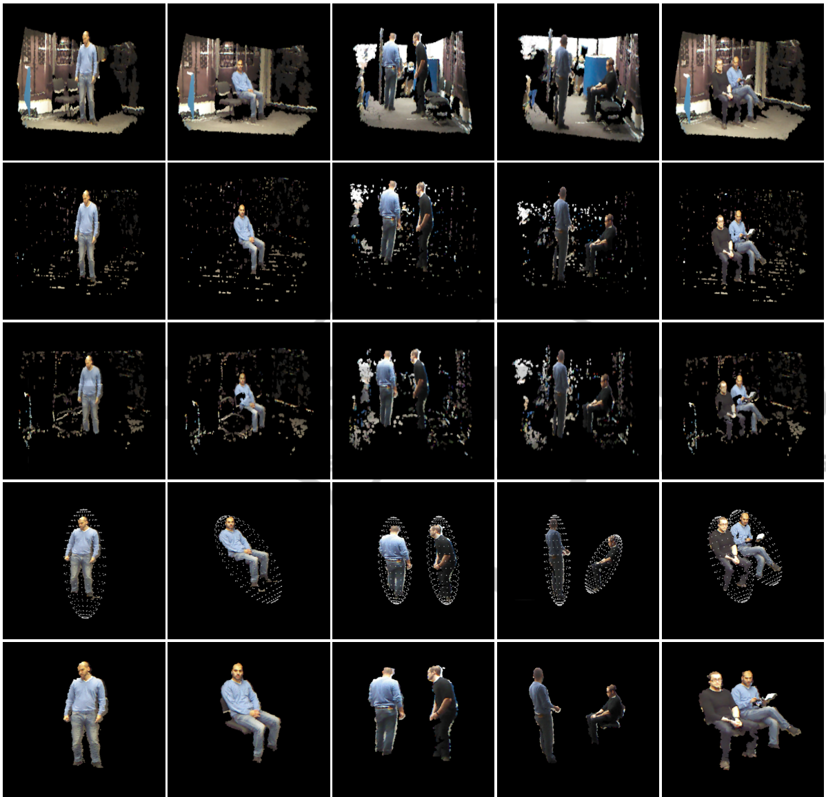
Figure 5: From top row to bottom: raw point clouds from different scenarios; foreground masks extracted by (Kammerl et al., 2012) approach; results from cloud to cloud background subtraction using a global threshold; The foregrounds extracted by our approach together with their encapsulated ellipsoids; ground truth masks generated by the implementation of (Shotton et al., 2013) in the OpenNI framework.
