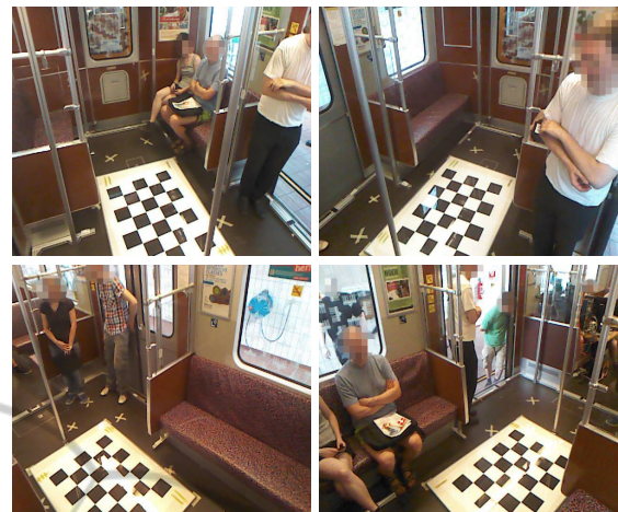
Figure 4: Regular chessboard used as a reference system for all sensors mounted in the train wagon.
