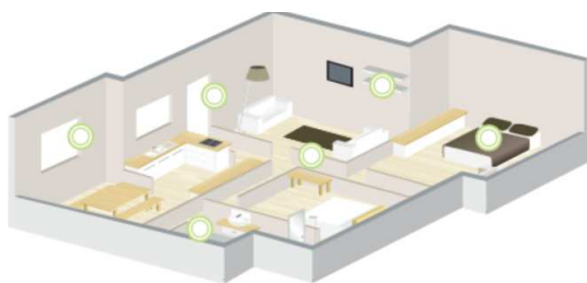
Figure 1: Schematics of living area of a senior. Circular icons are used to show various locations where on/off or proximity switches can be integrated into the living area.
