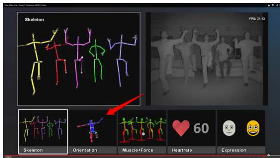
Figure 6: An example of sensing the movements of people through Kinect II sensor and various examples of the visualization of such movements.
