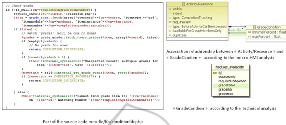
Figure 4: An example about relationship verification between the “GradeCondition” class and the “Activity/Resource” class.
