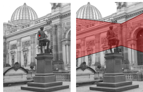
(a) One keypoint of the source image (b) Respective search region in target image
