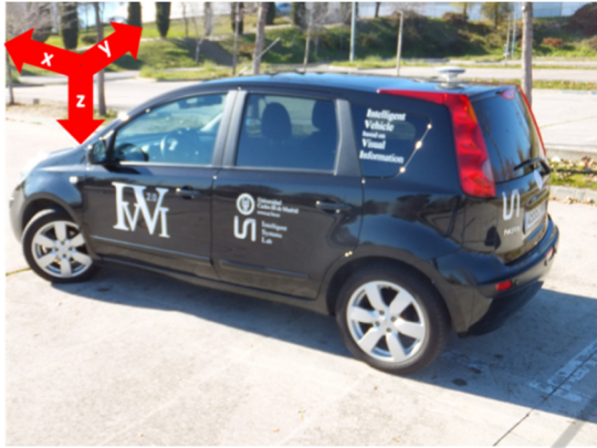
Figure 3: Axis representation: X=laser-obstacle distance, Z=detection height, Y=horizontal deviation.
