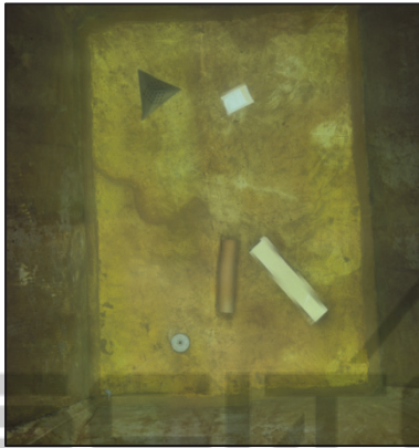
Figure 5: Image mosaic of the small pool at the Ocean Systems Lab obtained by registering and stitching the captured optical data.
