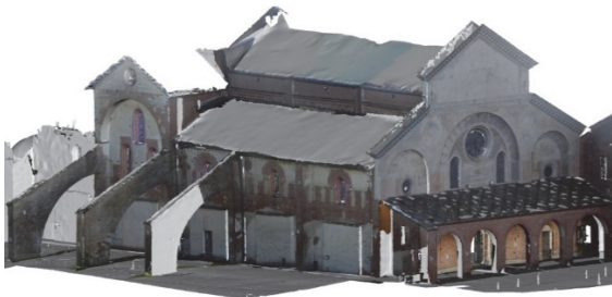
Figure 3: 3D Model processed from LIDAR data.
