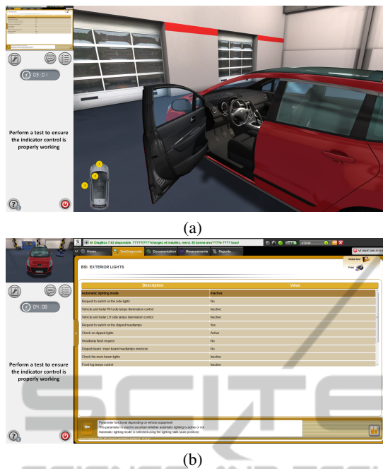
Figure 1: The game environment of Diag'Adventures features two views : (a) the interactive car in 3D and (b) the diagnostic software.
