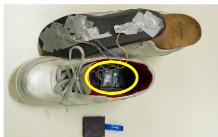
Figure 5: The shoe modified to host the wearable device: in evidence, the slot to accommodate the electronic board.
