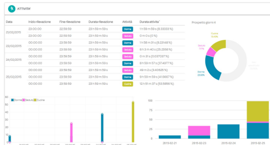
Figure 9: Screenshot of the remote platform interface showing presence graphs: each color represents the average time spent for the respective activity (blue for sleeping, green for cooking, magenta for sitting, grey for undefined).
