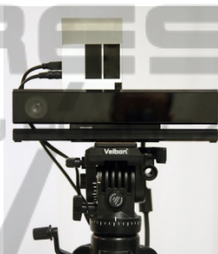
Figure 2: Argos P100 3D mounted on top of Kinect II.
