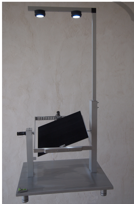
Figure 3: The constructed ball and plate system.
