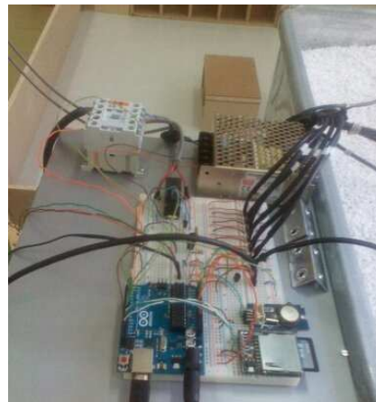
Figure 6: Control and data acquisition hardware built around an Arduino Uno board.
