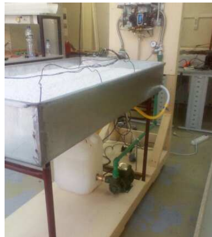
Figure 5: Detail on the water circulating system. Below the table it is possible to observe both the water pump and the reservoir.
