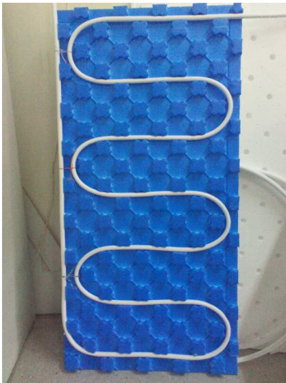
Figure 3: The growing stand internal piping system meander around a piece of styrofoam used in radiant floors domestic heating systems.
