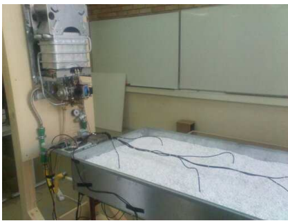
Figure 4: Distribution of the temperature sensors along the perlite.
