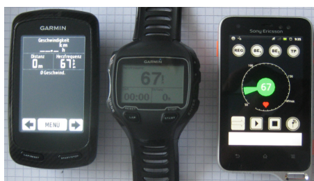
Figure 2: Two commercial sports units and one Android smart phone receiving the identical ANT+ signal from a heart rate chest strap. The left most device is for bicycling, the middle one is a Triathlon watch, and the smart phone was developed in a usability study on sports utilities.
