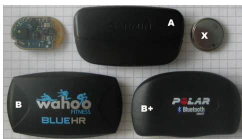
Figure 1: Body sensors for tracing sports and fitness activities. Upper left shows the circuit board of a footpod, while the other three devices are heart rate sensors. A works with the RF standard ANT+, while B and B+ are using Bluetooth as printed on their plastics case.
