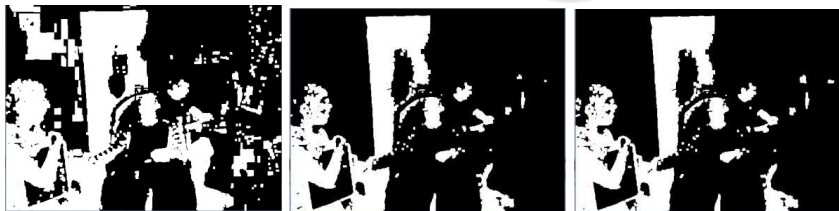
Fig. 13. Binarization obtained using different procedures: (a) Thr+EM, (b) Thr+Knn, (c) Thr+SVM. The data gathered by the previous methods is used later in the learning steps of classification methods like Support Vector Machines (SVM), Expectation-Maximization (EM), K-Nearest Neighbors (KNN) that will be used in the following subsection to segment images based on skin color.
