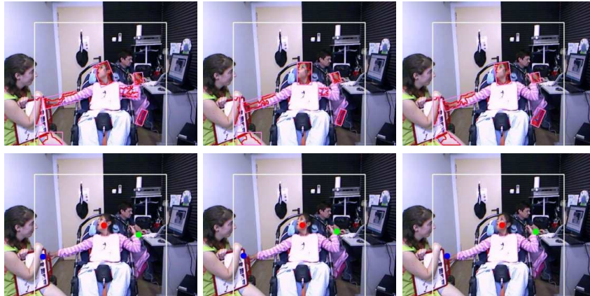
Fig. 17. Hand location and tracking. These images represent a sequence where detected regions are corresponded to head (red), left (blue) and right (red) hands.
