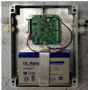
Fig. 3. Sensor node hardware, embedded into the terminals.
