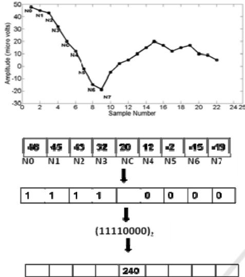
Figure 2: Computation of 1D local binary pattern.
