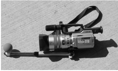
Figure 1: Camera used for the SFU Grey-ball dataset collection.
