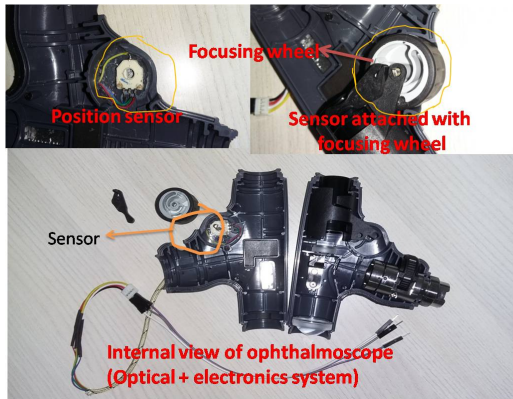
Figure 7: Housing of the position sensor inside the ophthalmoscope to measure the lens position. The sensor will measure the rotational movement ( \theta ) of the focusing wheel.
