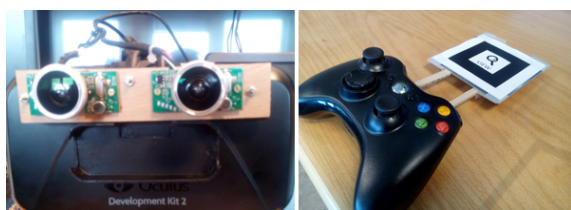
Figure 1: Left - the hardware rig consisting of an Oculus Rift DK2, dual web cameras and fish-eye lenses. Right - the marker-controller rig with custom made marker. By combining the two, both physical and virtual interaction can be achieved at the same time, while in the bird's eye augmented reality view.
