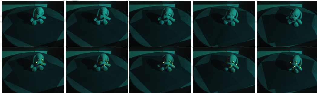
Figure 10: The visualized ground truth tracking data drawn on images of the 'Plush Dog' sequence. Top row: features generated by a grid within valid image region. Bottom row: features generated by SIFT method.
