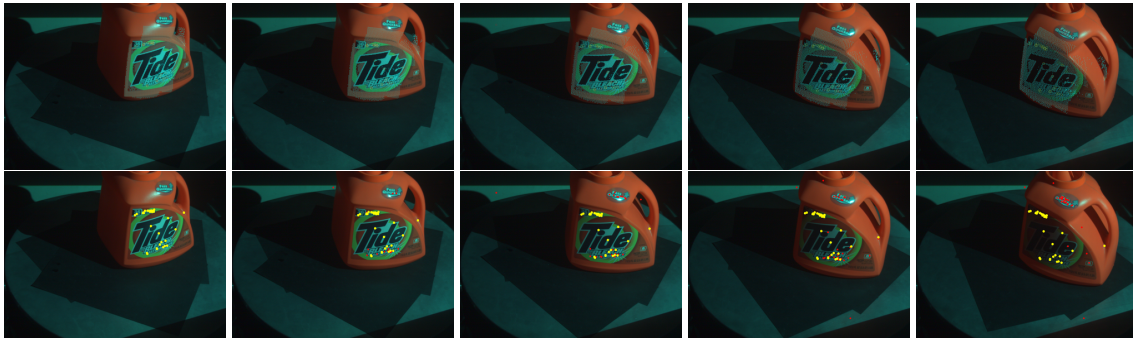
Figure 8: The visualized ground truth tracking data drawn on images of the 'Flacon' sequence. Top row: features generated by a grid within valid image region. Bottom row: features generated by SIFT method.
